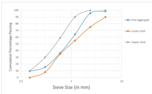
Figure 4 Particle-Size distribution of Fine Aggregate (Zone-II)
